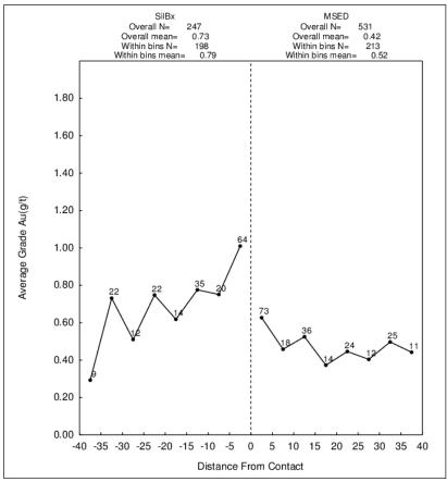
Figure 23: Contact Profile for Gold in Silicified Breccia Zone vs. Mineralized Sediments at El Capitan
