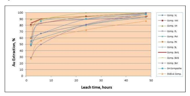
Figure 15: Medium Grind Bottle Roll Test Results
