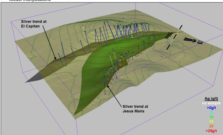
Figure 25: Interpreted Silver Trend Planes used to Control Dynamic Search Orientations during Model Interpolations
