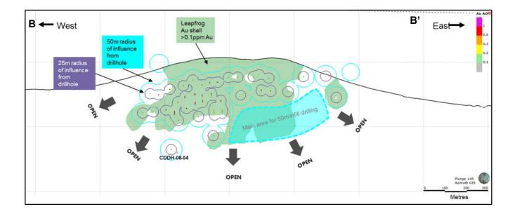
The long section is oriented with a plunge of +45 towards and azimuth of 039, perpendicular to the attitude of the mineralized zone. The long section shows the Leapfrog >0.1ppm Au shell, intersection of drill holes and radius of influence of 25- and 50-m around each drill hole to show for areas of gaps and potential for continuity of mineralization. Note zones for infill drilling, as well as for testing extensions downdip and on strike (Source: Riverside Resources Inc., 2019).
