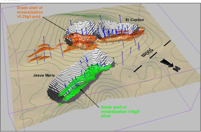
Figure 35: Isometric View of Grades Shells at Projected Cut-Off Grades Relative to Floating Cone Pit Shells
